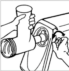
3. Loosen the screw plug on the right side of the mincer by turning it counterclockwise until you can take the worm housing out of the motor housing without any resistance (picture B).
