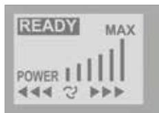
4. The display illuminates and you can see for 30 seconds ›Ready‹ blinking. ›Power‹, ›Max‹, 6 bars in different length, 6 arrows (3 pointing to the right and 3 pointing to the left side) and a rotating symbol (picture A) are indicated in the display. After 30 seconds only ›Ready‹ is shown in the display.
