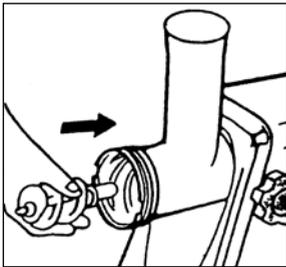
2. Insert the worm with the longer, narrower end into the worm housing and turn slightly until it is securely seated in the worm housing (picture B). Make sure that the worm is placed completely in the inside of the worm housing. If necessary turn the worm a little bit to make it fit. If mounted correctly only round about 9 mm of the axis of the worm are visible outside of the worm housing.
