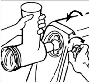
1. Loosen the screw plug on the right side of the mincer by turning it counterclockwise until you can fit the slim end of the worm housing all the way into the opening for the drive shaft. The opening of the worm housing should be upright (picture A). The worm housing is correctly mounted when the worm housing is flush with the motor housing. You should not be able to see the slim end of the worm housing anymore.
