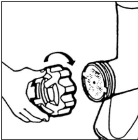
5. Firmly screw the closing ring on the worm housing and tighten by hand by turning it clockwise (picture G).
