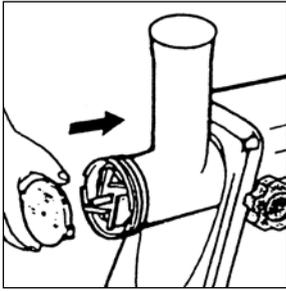
4. Mount the grinding disc on the knife. The arresting pin must lock precisely into the corresponding recesses (picture F).
